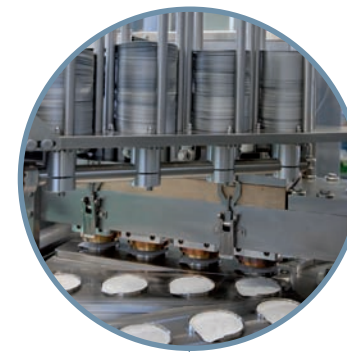
SELLADO MEDIANTE TAPA PRECORTADA O BOBINA DE FILM CONTINUO HEAT SEALING STARTING FROM A PRE-CUT LID OR CONTINUOUS FILM SPOOL THERMO SCELLAGE, EN PARTANT DE COUVERCLE PRÉ-COUPÉ OU BOBINE DE FILM CONTINU
