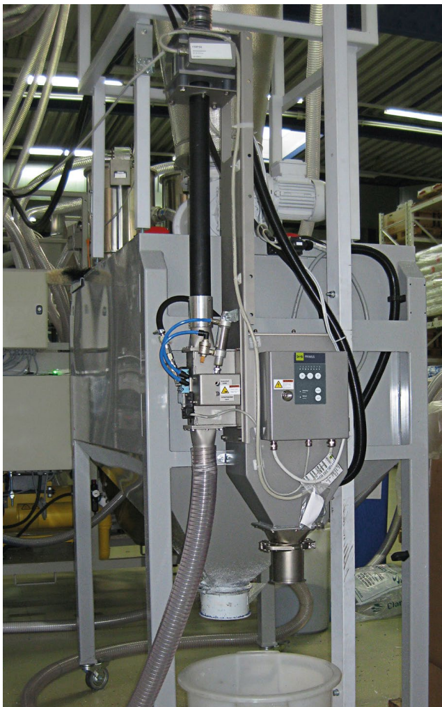
Installation example: Metal separator GF installed in a vertical pipeline (old version)
