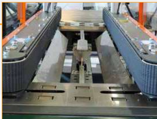
Folding system of bottom flaps (only HM11-TB)
