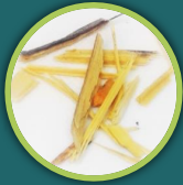
FB1 – Pallet wood splinter 12 x 3 mm
