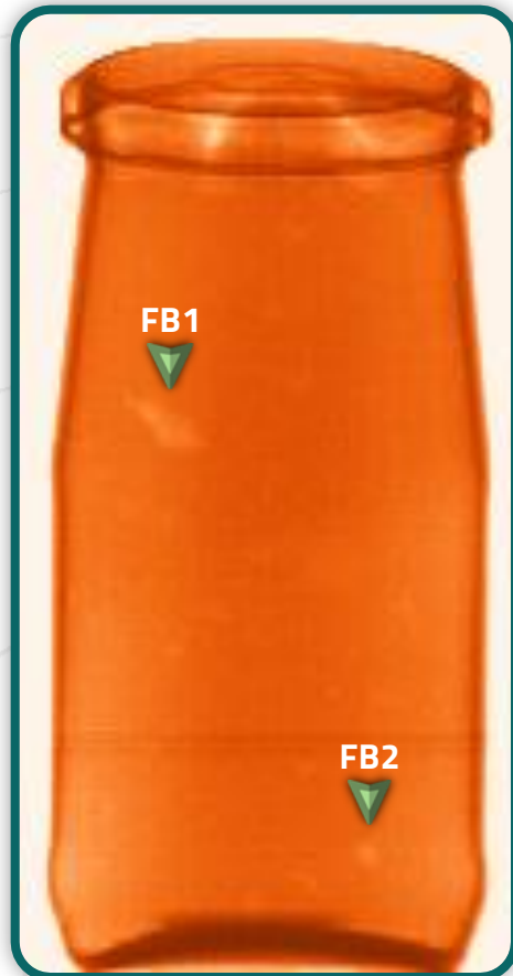
FB1 – Pallet wood splinter 10 x 4 mm
